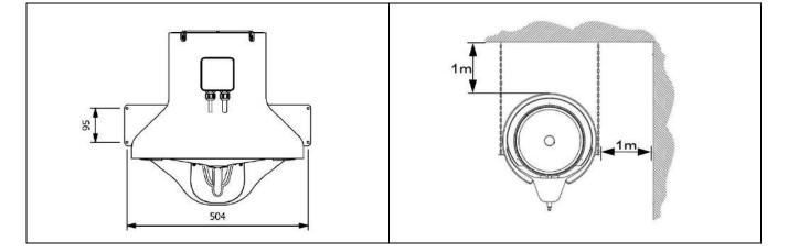
Fig. 2.2.1 - Fixing hole spacing and minimum wall distances
