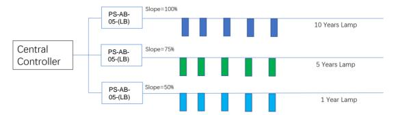
As the service life of the lamp is different, the output of the lamp will have light decay. Through the BluePotentionmeter, the brightness of different PS-AB-05-(LS) lights under the same central controller can be adjusted to ensure that the brightness of the farm is consistent and uniform.
