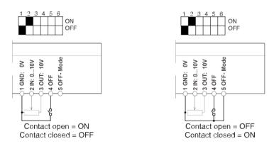
The ON/OFF function described naturally applies to all types of drive (pot., voltage source, sink current source) with DIP switch 2 at ON in each case.
