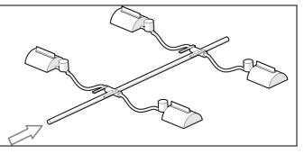
side is standard a 8 mm hose nipple (optional a smooth hose nipple or a G1/8" right handed thread. Other connections are possible after consultation). Always use approved gas sealant to close the gas connections.
