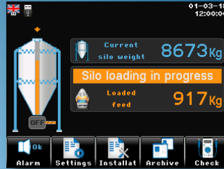
Viewing silo load
